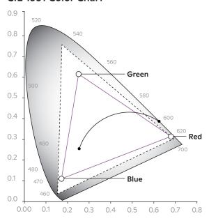
Ketra's A20 tunable lamp can easily be commissioned into Lutron HomeWorks or Athena systems. The product can reproduce any color point within the triangle shaped gamut indicated in the chart to the left. With Ketra's Color Lock tool, the color point is maintained to an accuracy of one-step MacAdam Ellipse over the lifetime of the product and across operating temperature range.
